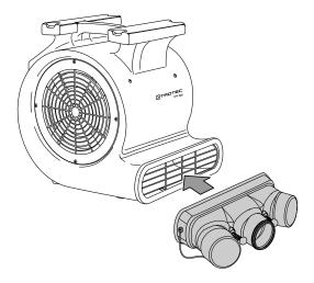
2. Move the attachment hooks around until they are hooked into the air outlet grille.
